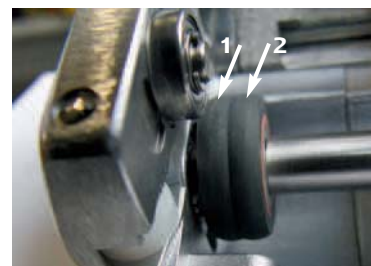
① Redundant friction wheel
