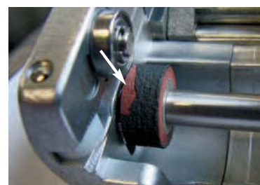
② Marking for wear and tear on the friction wheel red = exchange necessary
